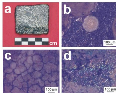
Figure 3. Images of some Medieval stained glass samples. External surfaces. (a) Bulk coloured violet glass as-received in the laboratory. (b) Crater, OM. (c) Crust formed by insoluble deposits, OM. (d) Small craters and insoluble deposits, OM
