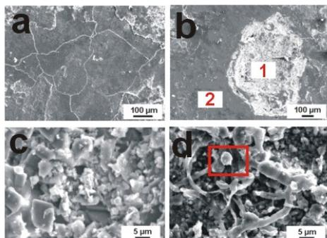
Figure 4. SEM micrographs of some Medieval stained glass samples. External surfaces. (a) Microcracks. (b) Crater. (c) Crust with calcium sulphate crystals. (d) Filament-like and spherical microstructures derived from fungal colonisation
