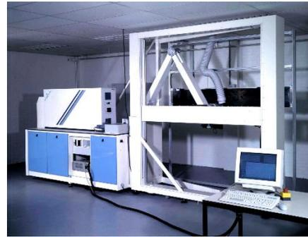
Figure 3. Laser workstation for cleaning of painting
