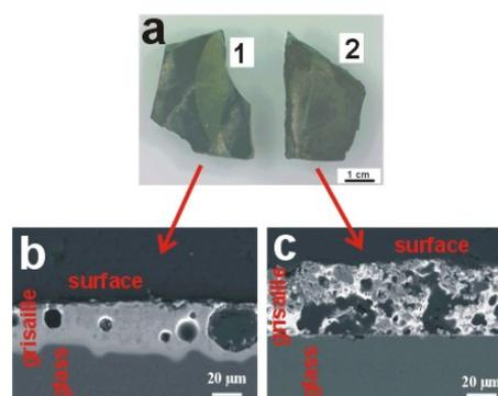
Figure 5. Images of some grisailles on Renaissance stained glass pieces. (a) Internal surface of two fragments with a dark brown grisaille as-received in the laboratory. (b-c) Cross-section SEM micrographs showing the glass, the grisaille and its external surface
