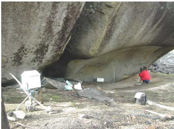
Figure 6. Nursery Swamp rock shelter showing the monitoring equipment used to determine environmental factors in relation to the growth of lichen
